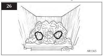
9.9 Place another two medium size coals resting behind the first three coals and against the flame baffle, Diagram 27.
